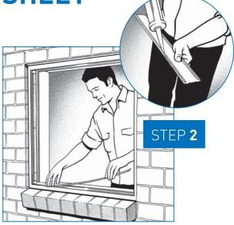
You have a number of long PVC strips the width of the frame and these sit under each course. Take one of these PVC strips and apply a thin bead of silicone down the shoulders of one side, then stick it to the frame at the bottom. Similarly, run silicone along the top to accept the first course of glass blocks. It does not matter which way around the PVC sits. Be tidy with silicone – wipe off any mess straight away.
