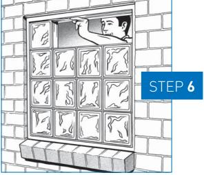
Continue to lay up to the top row where you again work from the sides towards the last glass block in the middle. In the last course a siliconed PVC infill is slid along between the frame and the top of each block as it is laid.
