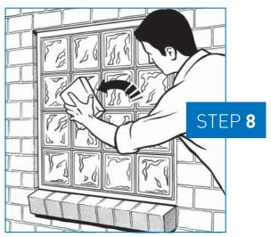
Grout the same as for tiles making sure you fill all the voids and compress the grout tightly in the joint. Clean off the excess grout with a damp sponge. Rinse the sponge continually so that any grit will not scratch the faces of the blocks. Squeeze the water out of the sponge so that the grout is not washed out. Leave to dry and then dust off with a cloth. Now enjoy your handiwork.
