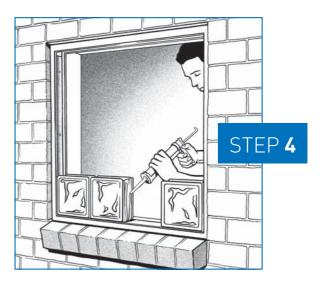
Once the bottom PVC strip and side PVC infills are stuck to the frame and silicone is on the inside of the PVC strips then you can start laying the glass blocks. Start at the bottom corners and work towards the middle of each course. Keep to the principle that all surfaces that come into contact have silicone so they stick together.
