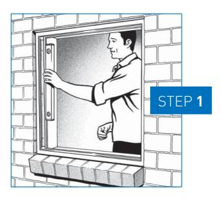
Install the frame securely into the opening using nylon anchors or similar simple fixings about every 400mm up the jambs. The frame must be plumb, level and squared.
